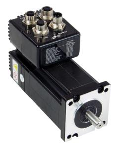
Applied Motion designed the STM/SWM integrated stepper motor package with the efficient and flexible positioning required by the conveyor system. Combining a motor, drive and control in one package, the STM/SWM incorporates an encoder with capabilities for automatic stall detection and prevention. The built-in encoder provides feedback to the integrated controller on the motor's actual position and closes the feedback loop to avoid limitations associated with stepper systems.
